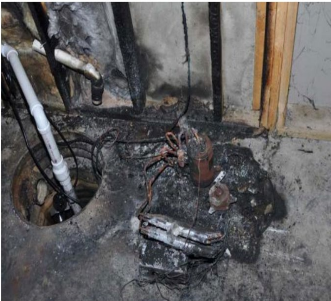
Figure 2: Photo of fire damage caused by a defective dehumidifier
